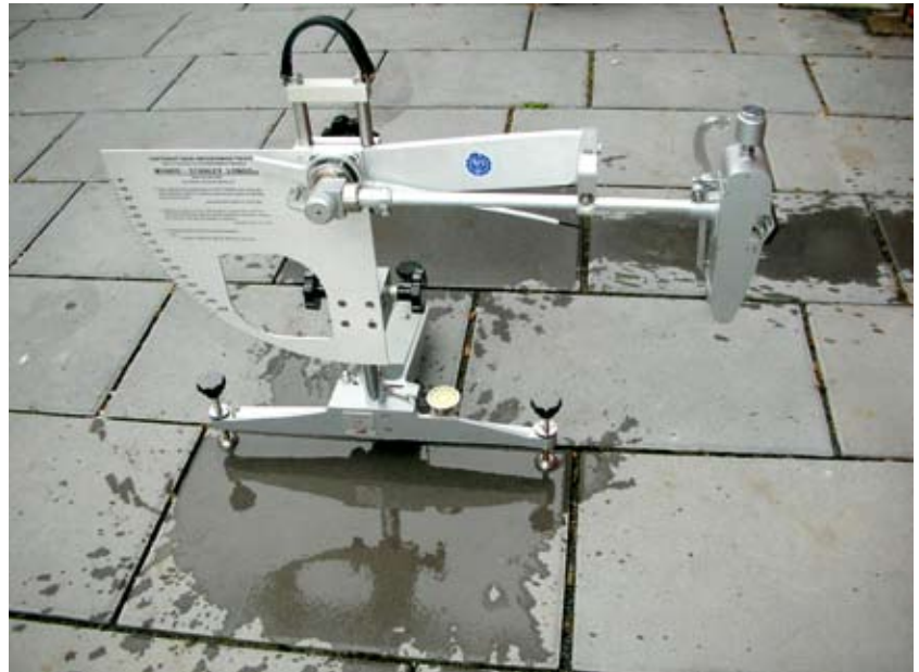
Fig. 1 Pendulum device to determine the sliding resistance value in accordance with [9, 10, 11].
