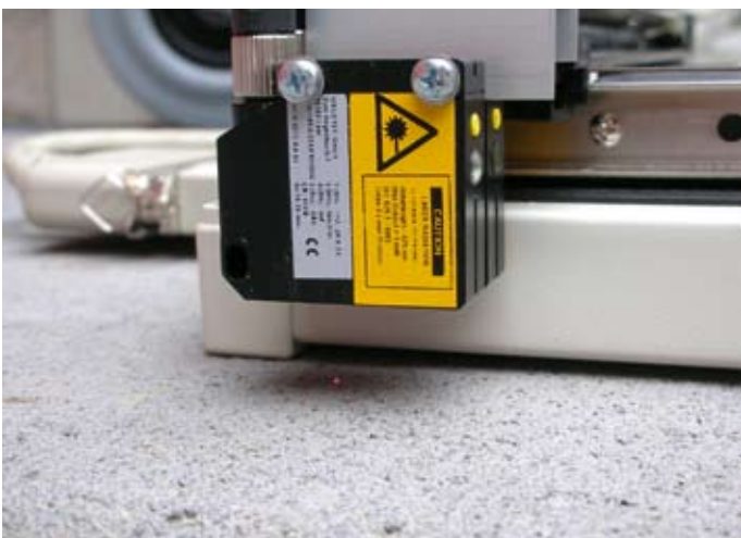
Fig. 3 Mobile laser system to measure roughness.
